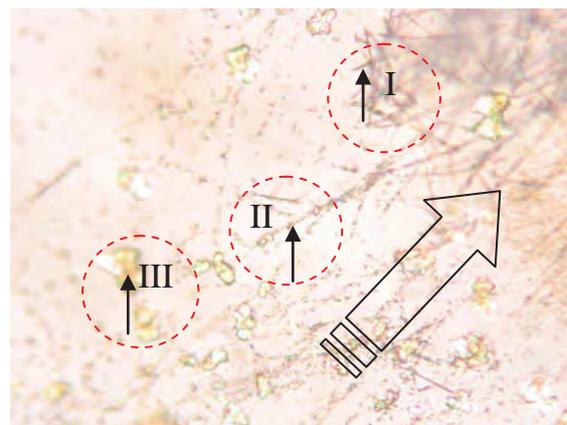
Fig. 2. Three phases of PRX release and crystallization. Light microscope image (magnification 50x) validating the results in Fig. 1. I. PRX inside the nanofibers is in amorphous state. II. Crystallization inside fibers. III. Recrystallization of PRX. The large arrow indicates the propagation direction of the water front.
