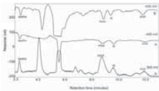
Figure 2: (A) Chromatograms of artificial plasma sample obtained at 500 and -400 mV. The sample was spiked with approximately 8.5 µg/L of analytes. (B) Chromatogram of plasma sample obtained from healthy subject.
