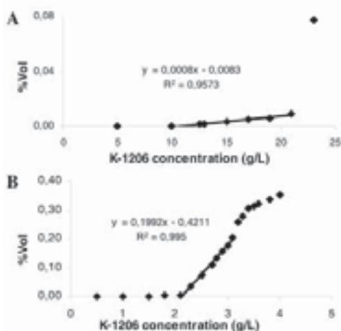
Figure 2: Measured %Vol vs K-1206 concentration in (A) alcohol and (B) mixture of 1:1 water and alcohol. The solid lines are linear fit to certain regions of concentration data.
