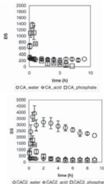
Figure 2: Swelling behavior of CA and CAC2 in different dissolution media
