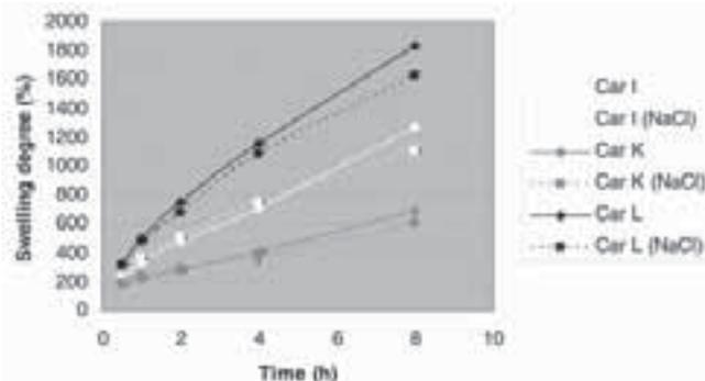
Figure 3: The swelling of different carrageenan matrices in media with and without NaCl. K represents kappa, I iota and L lambda carrageenan (Car). The data are means ± SD of 6 measurements.
