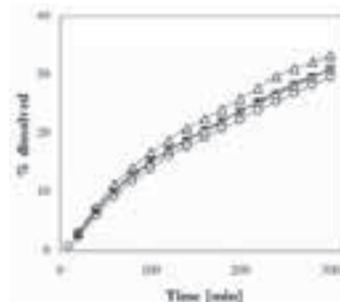
Figure 2: *In vitro* dissolution profiles at selected gastric residence times; 10 min (open circles), 40 min (squares), and 120 min (triangles), and predicted *in vivo* dissolution profile (filled circles).
