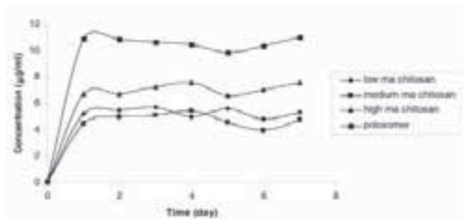
Figure 1: In vitro release profiles of triclosan from the grafts
