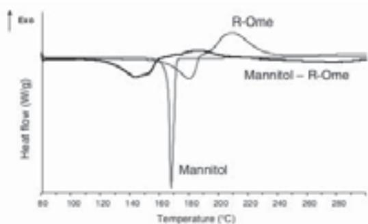
Figure 1: DSC thermograms of pure R-omeprazole (R-Ome) and mannitol and R-omeprazole-mannitol(Mannitol-R-Ome) mixture (50:50), (heating rate of 0.5 C min<sup>-1</sup>).
