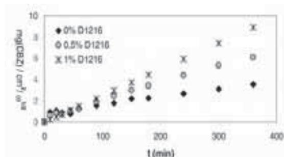
Figure 1: Intrinsic dissolution rate of carbamazepine in pH 9.0 with/without D1216
