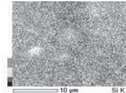
Figure 3: Surface distribution of montmorillonite by SEM EDS.
