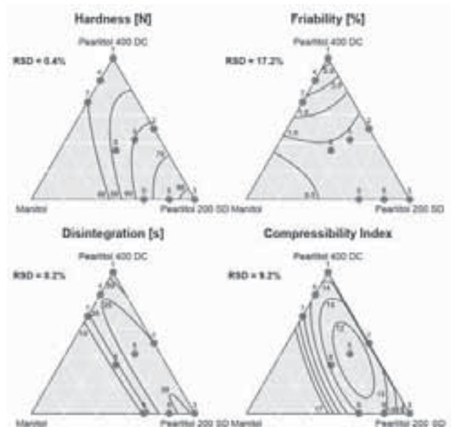
Figure 1: Fitted response surfaces represented by lines of constant hardness, friability, disintegration time, and compressibility.
