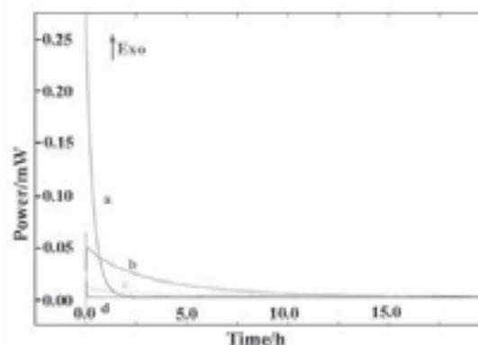
Figure 1: Power-time curves for the oxidation of methionine in (a) 0.3%  $H_2O_2$  solution; (b) 0.03%  $H_2O_2$  solution; (c) 0.003%  $H_2O_2$  solution; (d) water solution.
