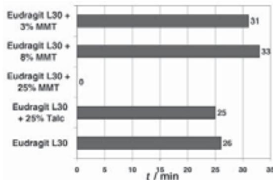
Figure 2: Disintegration time of coated tablets (Phosphate buffer 37 C, pH=7.2) after stirring 2 hours in HCl solution.
