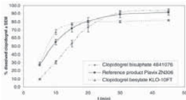
Figure 3: Comparative dissolution profiles of Clopidogrel bisulphate, Clopidogrel besylate and Plavix in FaSSGF, 500 mL, paddles, 50 rpm.
