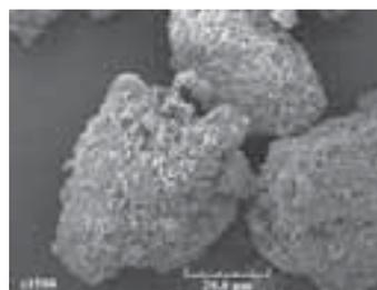
Figure 1: API microparticles trapped onto lactose granules
