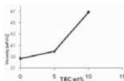
Figure 4: Effect of plasticizer inclusion on polymer coating dispersion viscosity.
