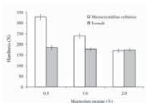
Figure 2: The impact of lubricant amount on the tablet hardness
