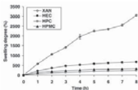
Figure 2: Swelling degree of different polymer matrices as a function of time
