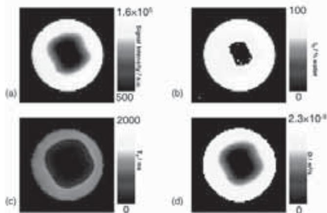
Figure 1: (a) a 64 × 64 RARE horizontal image taken through the HPMC/water system; the corresponding (b) water concentration (I<sub>0</sub>) map; (c) T<sub>2</sub> map; (d) diffusion coefficient map
