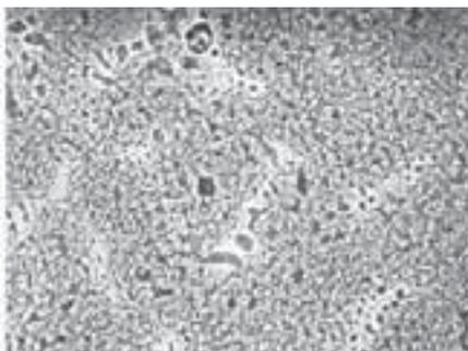
Figure 2: Ascorbyl palmitate nanosuspension after 5 cycles of ball milling
