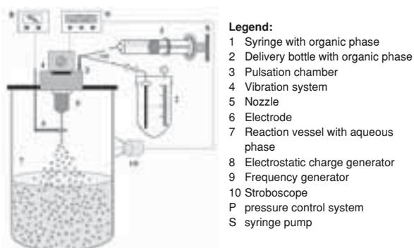
Figure 1: A schematic drawing of the NP production process.
