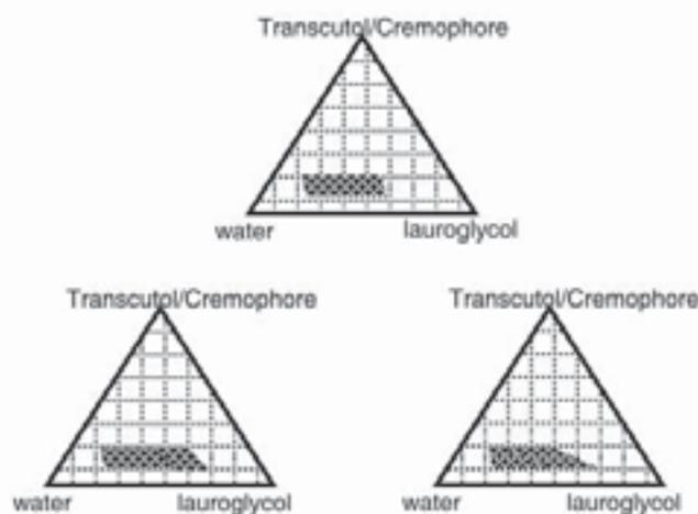
Figure 1: Pseudo-ternary phase diagrams indicating the efficient self-emulsification region (a-transcutol/cremophore ratio 1:1 (w/w); b-transcutol/cremophore ratio 1:2 (w/w); c-transcutol/cremophore ratio 2:1 (w/w)).
