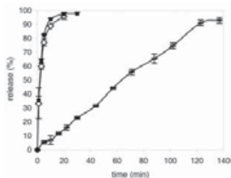
Figure 2: Dissolution profiles of:  $\diamond$  SNEDDS pellets A;  $\blacksquare$  SNEDDS pellets B;  $\blacktriangle$  piroxicam
