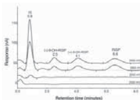
Figure 1: A typical chromatogram obtained after spiking medium quality control sample. RISP and both 9-OH-RISP enantiomers concentrations were 10.2 and 6.8 ng/mL, respectively.
