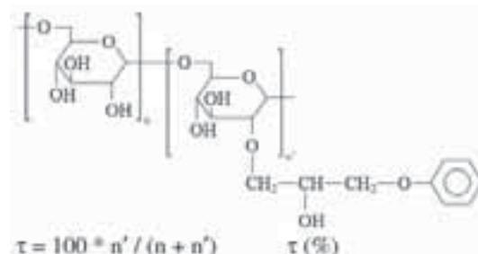
Figure 1: dexP and substitution degree ( $\tau$ )
