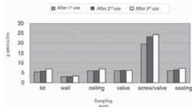
Figure 1: The residue of amoxicillin after three consecutive uses of the same container (granules case)
