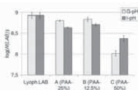
Figure 2: Resistance against acid conditions (G-pH; bright columns) and final survival after tablet disintegration in a fluid of intestinal pH (I-pH; dark columns) regarding the excipient ratios (see Table 1).
