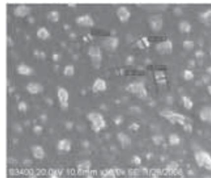
Figure 2: SEM of repaglinide loaded SLNs
