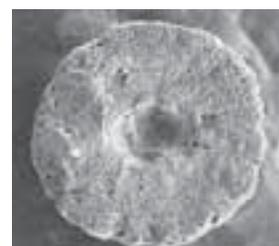
Figure 1: SEM micrographs section of pellets from experiment E at 140 X magnification (Zeiss Supra, 35 VP)
