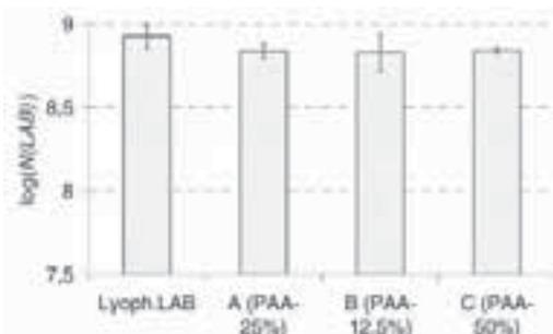
Figure 1: Survival of LAB after constant compaction force (0.5 kPa) and different excipient ratios (see Table 1).
