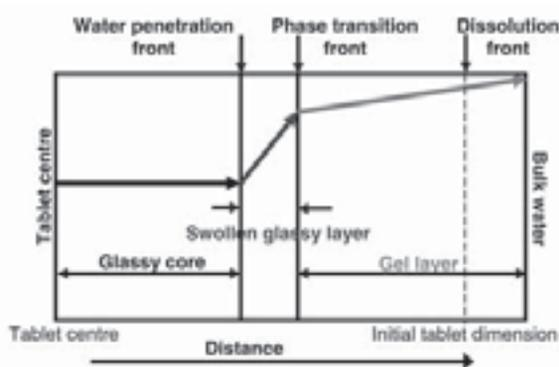
Figure 2: 1D schematic describing the phase boundaries of the swollen HPMC polymer in water
