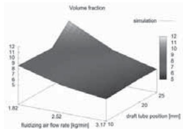
Figure 3: Volume fraction of pellets inside the Wurster draft determined by the simulation.
