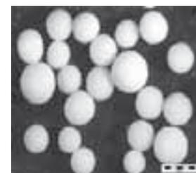
Figure 2: Surface of pellets from exp. E at 40 X magnification (Stereomicroscope Olympus)
