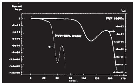
Figure 2: TSC curves of PVP and PVP+25% H<sub>2</sub>O
