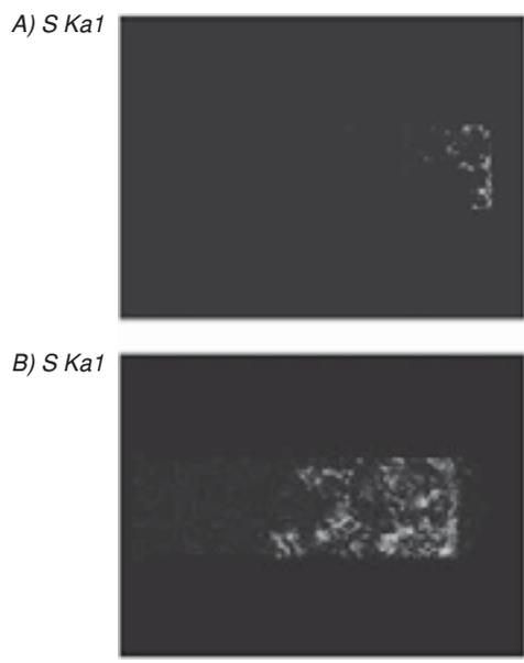
Figure 2: Depth of ZnS nanoparticles penetration measured with EDS analysis for tablets filled using megnetic stirrer (A) and ultrasound for one minute (B).
