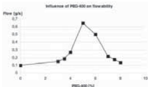
Figure 1: Effect of PEG-400 content on the flowability of powder mixture for briquetting.
