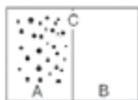
Figure 1: Dissolution of particles takes place in aqueous compartment A, then transported across membrane C to compartment B where it is accumulated.
