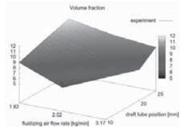
Figure 2: Volume fraction of pellets inside the Wurster draft determined experimentally.
