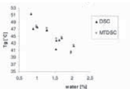
Figure 1: The effect of water content on Tg
