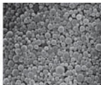
Figure 1: SEM images of PLGA microparticles.
