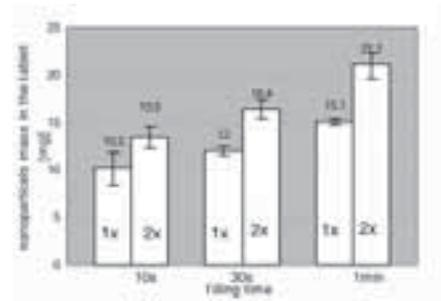
Figure 1: Mass of incorporated ZnS nanoparticles after first (1x) and second filling (2x) using different sonication time.
