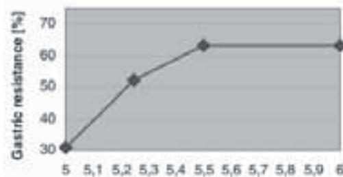
Figure 2: Influence of degree of neutralization on gastro-resistance of coated pellets
