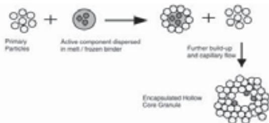
Figure 1: Schematic illustration of an encapsulated granule formation process by the immersion and layering mechanism.
