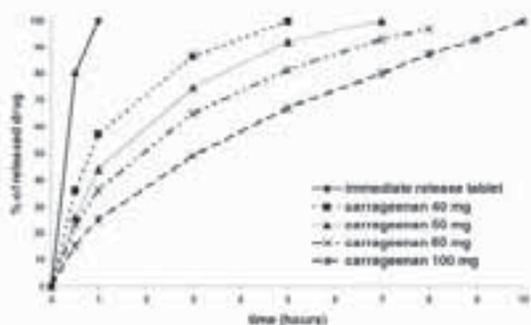
Figure 1: Drug release from the carrageenan containing matrix as a function of polymer content
