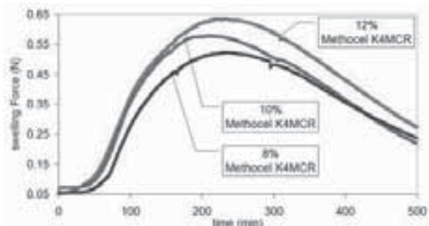
Figure 1: Swelling force of gliclazide tablets with Methocel K4M CR content of 12 % per tablet, 10% per tablet and 8 % per tablet.
