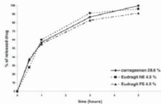
Figure 3: Comparison of drug release from carrageenan matrix tablet and polyacrylates reservoir system
