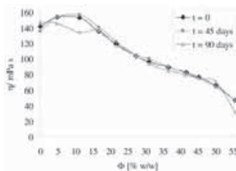
Figure 1: Dynamic viscosity of selected microemulsions as a function of the water ratio after 0, 45 and 90 days storage at 40 °C.
