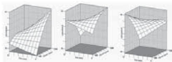
Figure 1: The influence of mixing time (x-axis) and mixing speed (z-axis) on the useful yield (y-axis) at three different binder concentrations.
