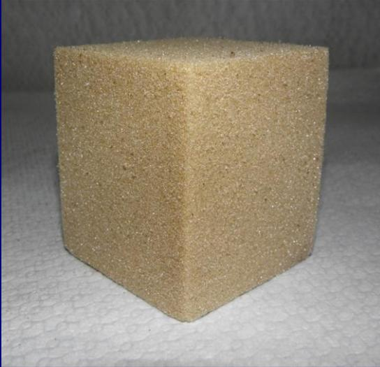
Polyurethane foams based on liquid wood polyols,
